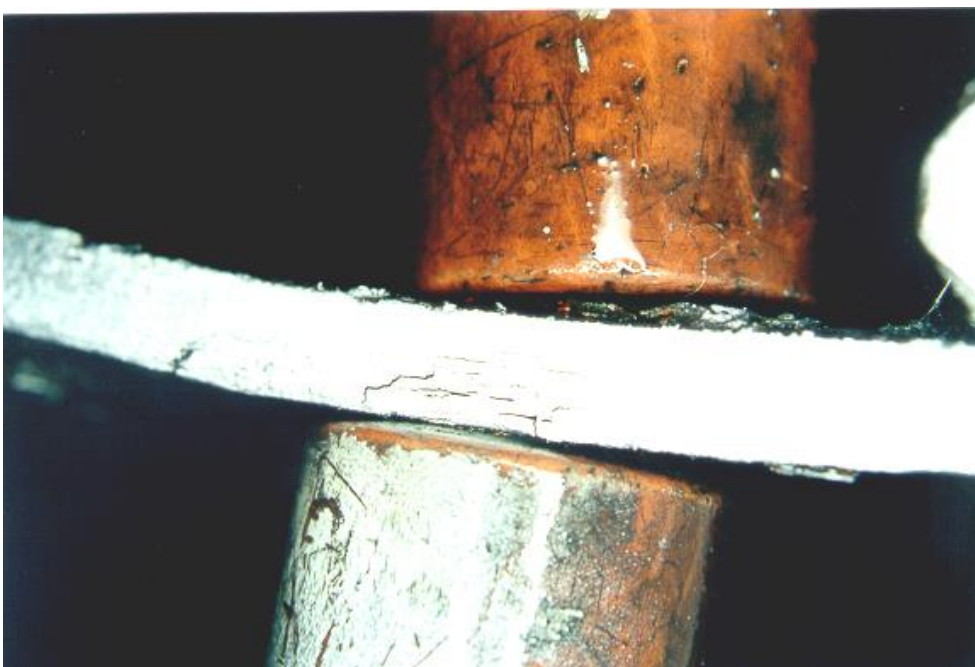
Figure 15 - Web edge filed and mpi, showing laminations clearly, positively identifying wrought iron
