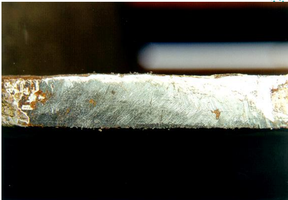
Figure 16 Edge filed prior to mpi. Laminations just visible
